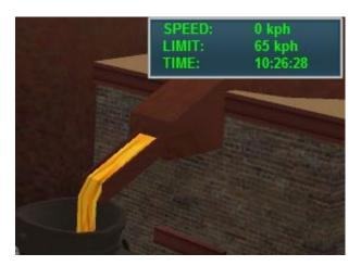
10 minutes after the slag and hot metal have emptied the recharging of the furnace with ore, coke and limestone using the suspended skip on the gantry crane will commence.
